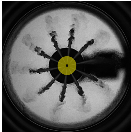
Figure 3.11: The area marked with the color overlay used to compute the background subtraction for the detection of the first sight of fuel.
