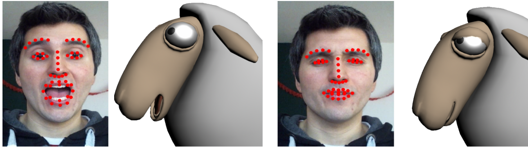
Figure 8.9: Examples of facial motion transfer learned from 6 correspondences. The first and second columns: Face and the second and fourth columns: the synthesized Sheep .
