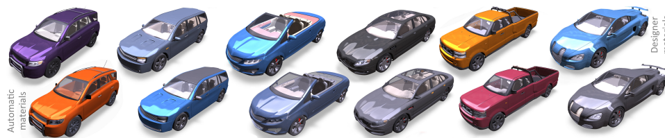
Figure 6.6: Automatic material assignment: database of cars where the materials are assigned by a human designer (1st row), results of automatic material assignment (2nd row). Results are generated by leaving out the particular query car from the database.
