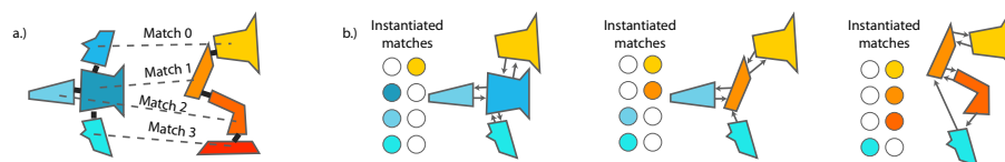
Figure 5.10: Finding contacts for interpolated shapes: a. ) for the source shape and the target shape it is known which nodes are in contact by the shape analysis; b. ) to generate an interpolated version between the source and the target shape, either the node from the source or from the target shape can be instantiated for each match. An instantiated node wants to connect to its contact partners that originated from the same shape; however, if a contact partner is not available, a node connects to the node of the other shape with which the original contact partner forms a match.
