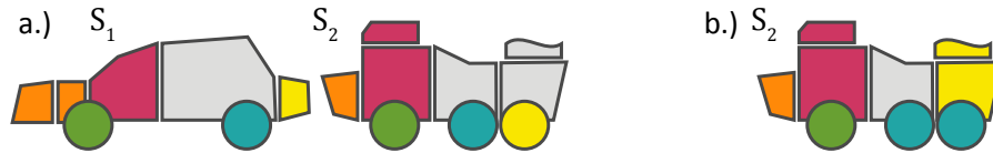
Figure 5.6: Re-grouping parts (represented by polygons) into nodes (represented by the same color) of a new hierarchy can help to find a better match between two shapes S_1 and S_2 : a.) original hierarchy for both shapes; b.) updated hierarchy of the target shape S_2 .
