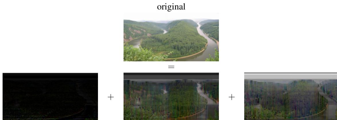
Figure 1.1: Decomposition of an image for CMLA2 such that every two rows of the double parts (the two images on the right) have the same content and the sum of all row maxima is minimized. The singleline part is the almost completely dark image on the left.
