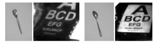
Figure 2.20: Reflections at the inner side and at the outer side of a spoon, taken from a distance of 5 meters. The 18 px font is readable from the reflection in the right figure, and almost readable in the left figure.
