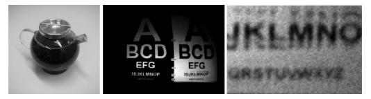
Figure 2.15: Reflections in a tea pot, taken from a distance of 10 meters. The 18 px font is readable from the reflection.
