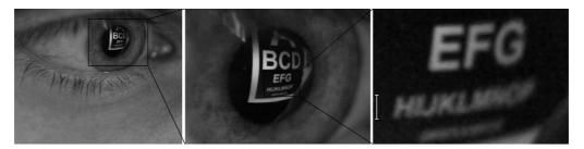
Figure 2.3: Image taken with a macro lens from short distance, where additionally the distance between the eye and the monitor was reduced. Readability is essentially limited by the camera resolution.
