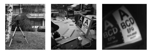
Figure 2.21: The attack in-field. The distance between the telescope and the office was approximately 18 meters (left), the desk where the monitor shows our test image (middle), and the captured reflections (right).
