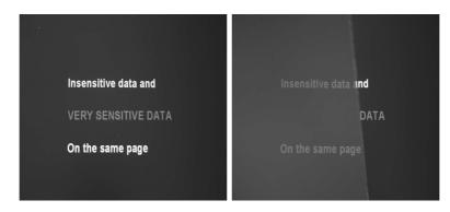
Figure 2.35: Image of the protective filter in front of a monitor showing sensitive information in blue color and insensitive information in white color. The left side shows the monitor without filter, the right side shows the monitor where the filter is applied to the left 2/3 of the monitor.
