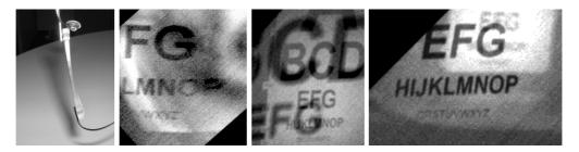
Figure 2.17: Reflections in eye-glasses, taken from a distance of 5 meters. Both the inner side and the outer side of glasses produce reflections. The 18 px font is readable from the reflection.
