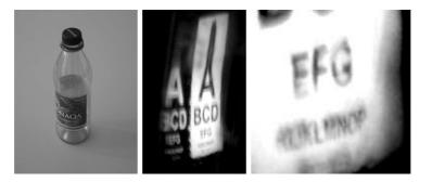
Figure 2.13: Reflections in a 0.5 l plastic bottle, taken from a distance of 10 meters. The distortions are caused by the irregular surface of the bottle.
