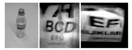
Figure 2.19: Reflections in a 0.5 l plastic bottle, taken from a distance of 5 meters. Because of the irregular surface, only parts of the text are readable.
