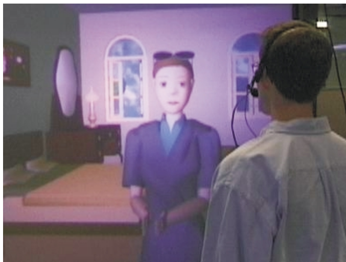
Figure 4.3: In the REA system, a virtual real-estate agent interacts with the user using conversational gestures.
