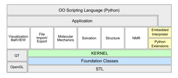
Figure 6.1: Overview of the structure of BALL. The basic components are in white, the scripting language support in yellow and external libraries that are not part of BALL are in gray.
