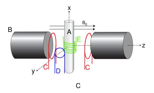
**Figure 4.2:** Basic components of an NMR spectrometer: The sample (A) is placed in a strong homogeneous magnetic field  $\vec{B}_0$  caused by a magnet (B). The field can be modified using the sweep coils (C). Radio pulses are transmitted using the transmitter coils (D) and received via the receiver coils (E).
