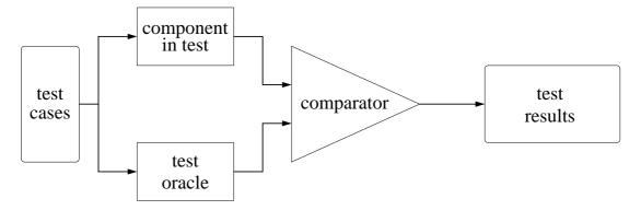
Figure 7.2: General software testing scheme
