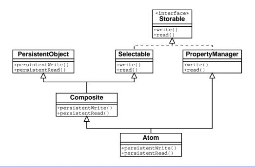
Figure 6.5: The Atom class and its base classes.
