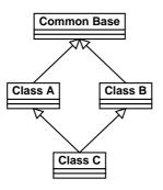
Figure 6.3: Multiple inheritance: the "deadly diamond"
