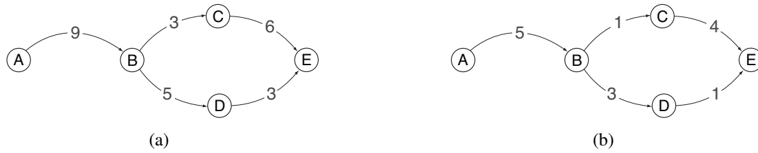
Figure 3.3: The (a) initial and (b) final state of the credit network with a credit payment along multiple paths. A pays 4 credits to E : 2 credits are paid along the path A \rightarrow B \rightarrow C \rightarrow E and 2 credits are paid along the path A \rightarrow B \rightarrow D \rightarrow E .
