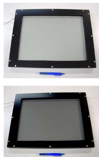
Fig. 7: Bleached and grey colored EC window of the INM (size 400 mm x 300 mm). The transmission in the visible range (TL value, DIN EN 410) can be varied from 60 % (bleached) to 20 % (grey colored, voltage < 3 V, switching time 2-3 min).
