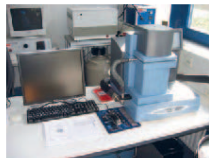
Figure 5: Dynamic mechanical thermal analysis setup for polymer matrix nanocomposite films and bulks.
