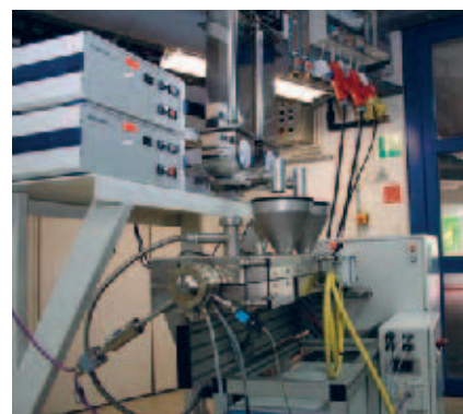
Figure 4: New two screw extruder for thermoplastic processing and compounding at the lab scale.
