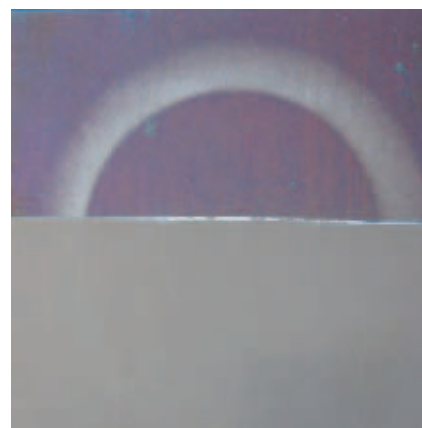
Figure 4: SiC coated steel sample after taber-abrader test.
