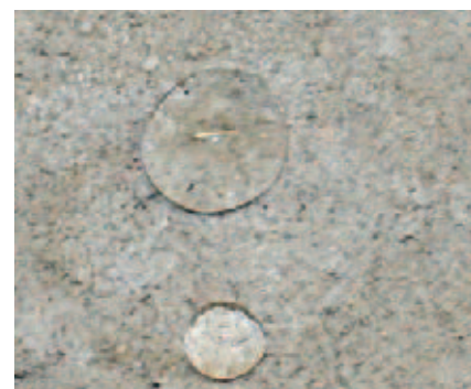
Figure 6: Hydrophobic effect of a surface of a concrete with INM additive.
