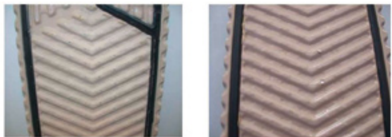
Figure 10: Heat exchanger plates coated with nanocomposite anti-adhesive systems after 4 h test in the heat exchanger at LUFA Norwest, left: epoxy nanocomposite EP A2, right: polyurethane nanocomposite PU A10
