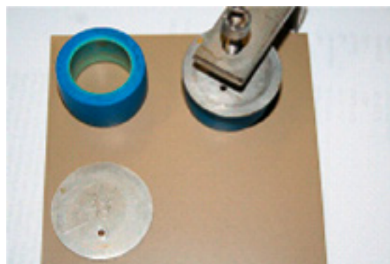
Figure 1: Experimental set-up for determination of chemical resistance of nanocomposite coatings: small pots filled with test liquid were fixed on the coated substrates and placed in a convection oven at 90 °C
