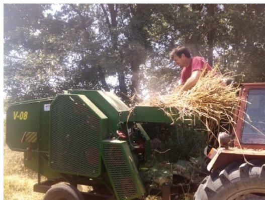
Fig. 1. Threshing wheat in a mobile threshing machine "ER-NET" Type V-08
