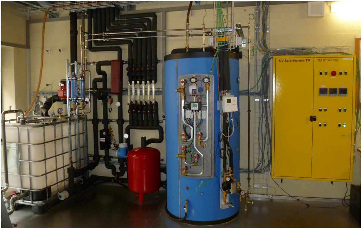
Fig. 5: Solar thermal Laboratory of the Institute of Energy Systems and Fluid Engineering (IEFE). Solar energy storage tank (blue), large reservoir as a reference for short term measurements (white)
