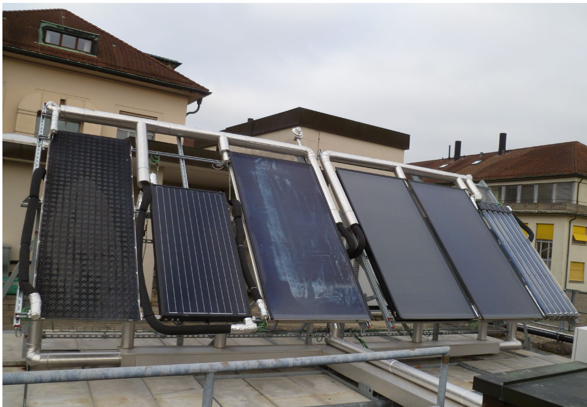
Fig. 4: Collector test field for lab experiments and student projects
