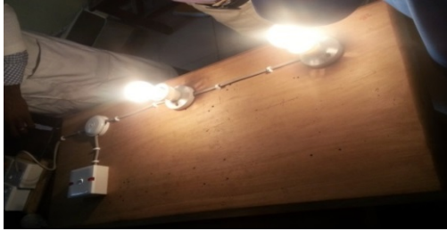
Fig. 9: Wiring of Lighting Points Serially
