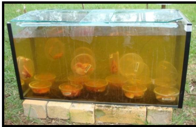
Figure 3.10 Set up of skeletal samples in fresh water and salt water tanks.
