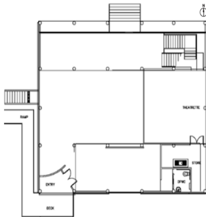
The ground floor of the hay shed following the adaptation.
