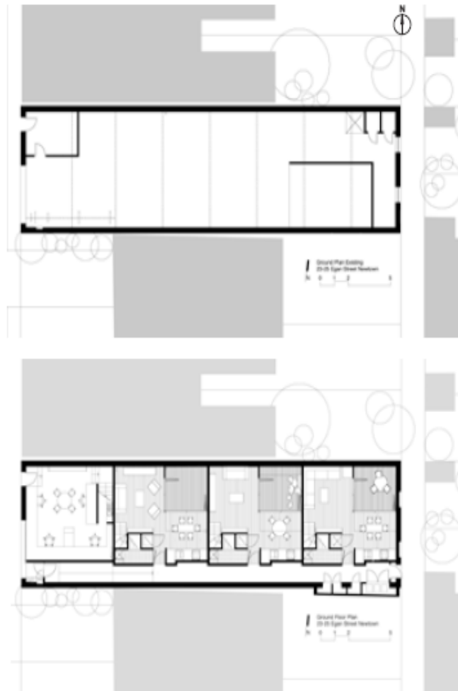
Above: The Industrial warehouse prior to adaptation. Below: The building after adaptation for apartments.
