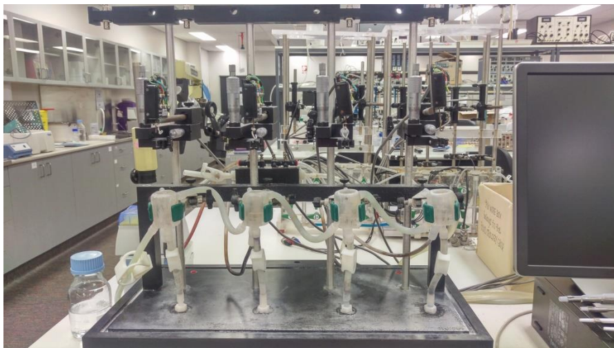
Figure 2.1 Set-up of four 8ml organ baths (EZ-baths, Global Towns, CA) with isometric transducers attached.
