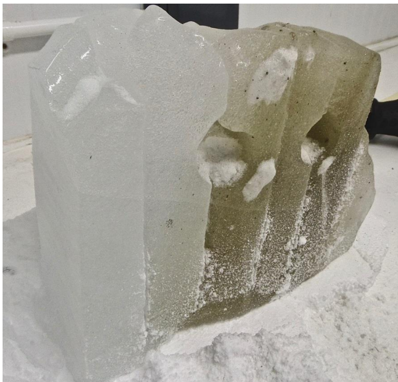
Figure 6 – Photograph taken during the second stage of blue ice sectioning. Each of columns were divided into six samples from different depths (note that the column pictured is turned on its side). The two large circular holes are remnants of the original sampling procedure. The variable colouration results from uneven levels of debris interspersed throughout the block.
