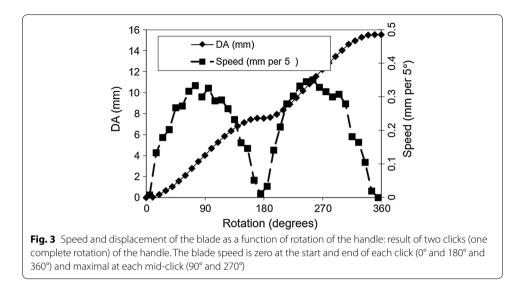
reverses slightly. This back drive is the basis of self-retaining action; after the back drive, the blades must be separated slightly to rotate the crank in either direction. However, the loaded tissues are forcing the blades together, thereby locking the rack-and-pinion in position. This mechanism, thus, produces a retraction speed that is highly non-linear, including brief moments of backward motion (Fig. 3).
