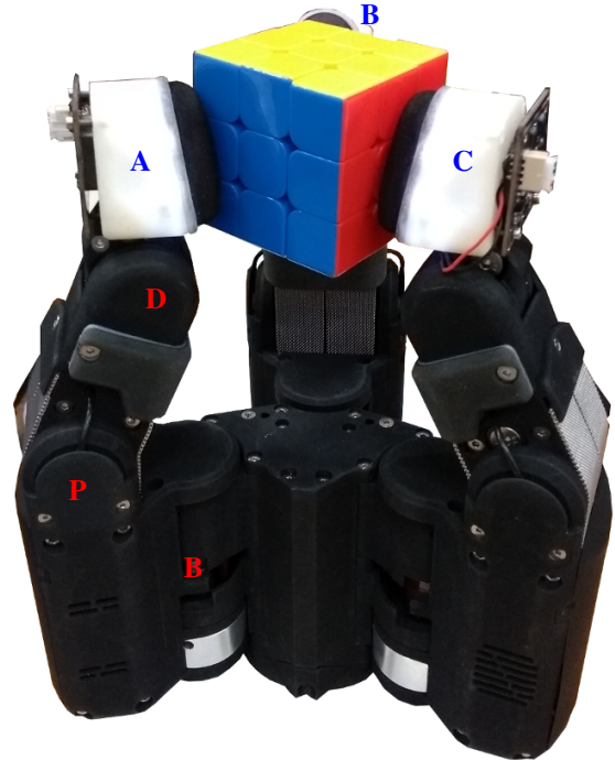
Fig. 1: Image of the developed tactile sensors integrated with the Shadow Modular Grasper. Base, proximal and distal joints are labelled in red, B , P and D respectively. Tactile fingertips A , B and C are labelled in blue.
