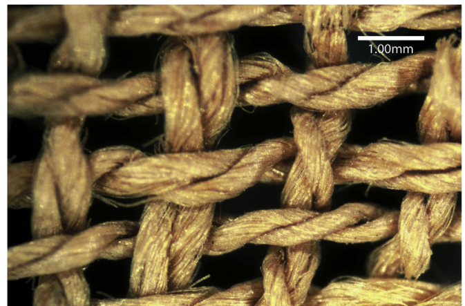
Fig. 4. Linen from basket, showing Z2S, a ‘prehistoric’ spin direction. Epi-darkfield.
