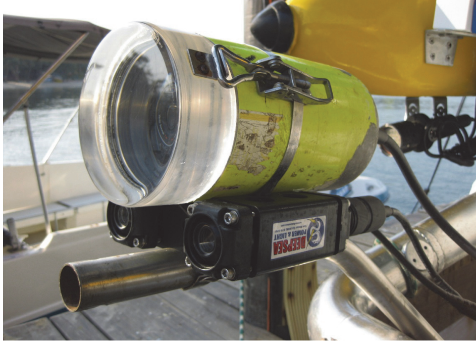
Figure 4. The laser mount (in black) is positioned below the camera housing (in yellow).
