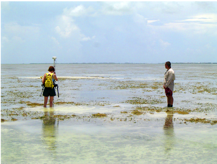
Photo 3. NOAA staff map the dimensions of vessel grounding injury features by walking the perimeter of each feature using Differential GPS. Photo by Amy V. Uhrin.
