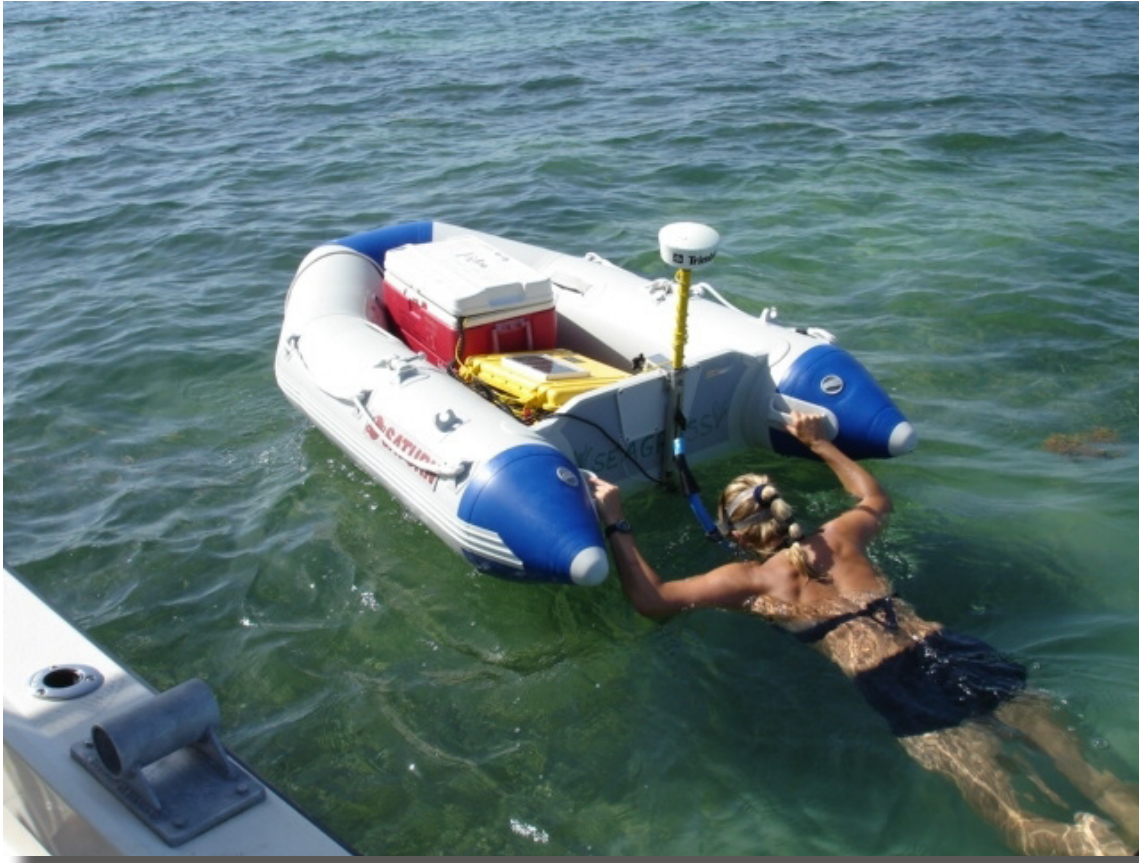
Photo 5. NOAA staff use a Lowrance LCX-15MT depth sounder integrated with the Differential GPS (mounted on the stern of an inflatable boat) to collect geo-referenced depth soundings (0.1 m vertical accuracy) within blowhole features. The boat is slowly guided back and forth across the injury on foot or via snorkel. The resulting bathymetry file is used to create a bathymetric grid layer enabling the calculation of blowhole volume (cubic meters). Photo by W. Judson Kenworthy.
