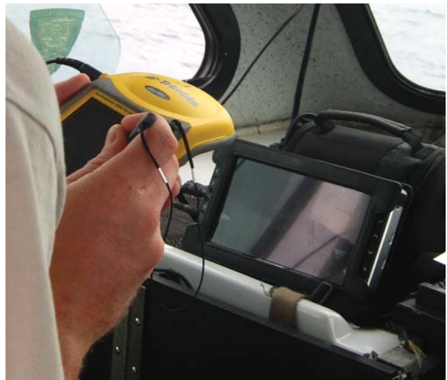
Figure 3.15. Topside field equipment used to collect georeferenced underwater video at GV and AA drop camera sites. While the SeaViewer unit was in the water, a field scientist logged positioning information and entered habitat data using a Trimble GeoXH GPS receiver while viewing real-time footage via a SeaDVR.
