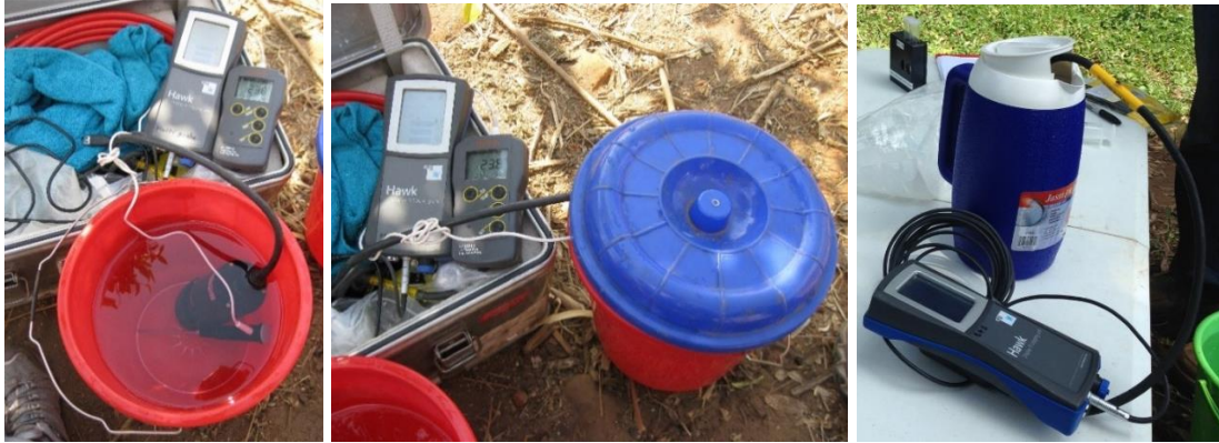
Figure 3.1 Left: TLF probe and clean thermometer in rinsing bucket. Middle: TLF probe and thermometer covered by lid and placed in shade for TLF reading. Right: TLF probe used in a clean dedicated smaller container with integrated lid [Jade Ward and Dan Lapworth/BGS]
