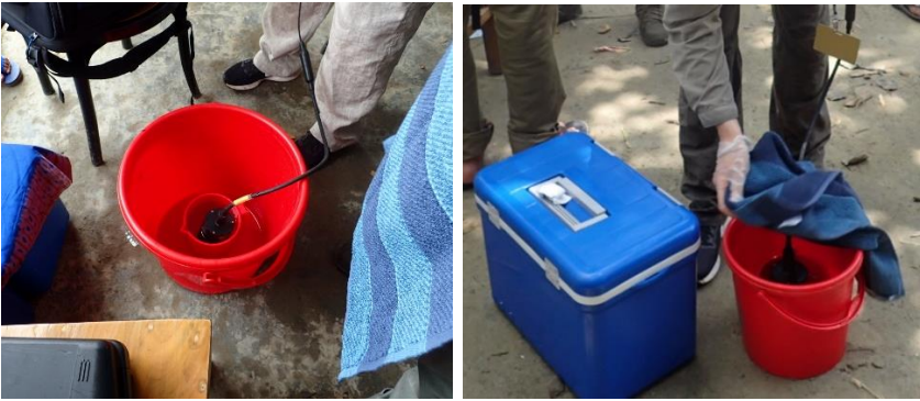
Figure 3.3 Left: arrangement of TLF probe with small beaker for taking measurements. Right: covering TLF probe with thick cloth to stop UV light interference [Saskia Nowicki/REACH]
