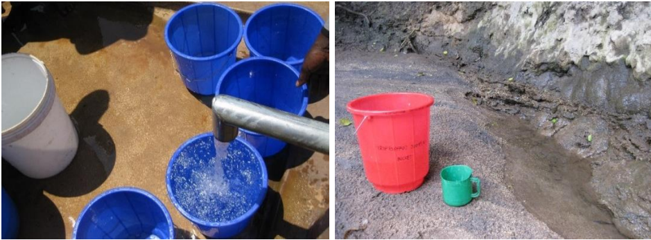
Figure 3.2 Left: Always fill the sampling bucket directly from the borehole spout or the bucket normally used for a shallow well. Right: for other sites such as for a dry river bed well use the sampling container which is normally used to draw water from the source [Jade Ward/BGS]
