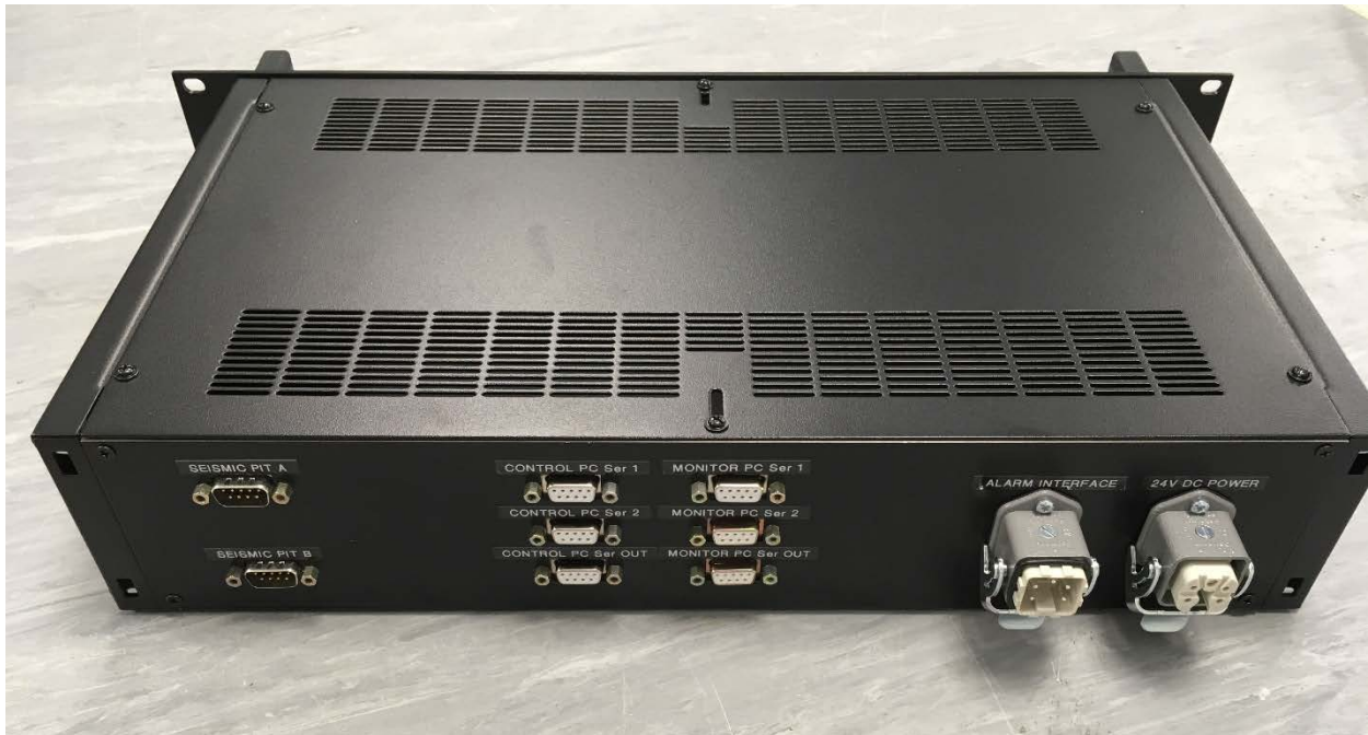
Figure 3. 'Alarm control unit' - rear view (serial port and alarm connections).
