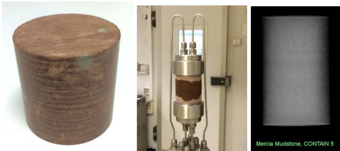
Figure 1. A sample of Mercia Mudstone after preparation (left), arranged within the isotropic test assembly (centre) and as a 2D x-ray image (right).
