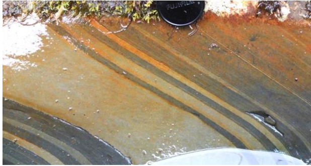
Figure 4A. Delicately laminated, anoxic hemipelagic mudstones (dark grey-black) with fine-grained sandstone and siltstone turbidite beds and laminae (pale grey/brown) (RO = 0; see Table 1) at c 1.32 m (see Figure 3). Lens cap is 5 cm in diameter. The thickest turbidite bed is 'flag G' of Jones (1909; see also Cullum & Loydell, 2011).
