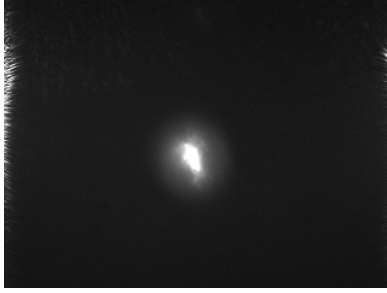
Figure 4.5: Infrared camera image of the MOT from our vacuum chamber. Fluorescence detected from the cloud of atoms trapped at the MOT centre can be seen.
