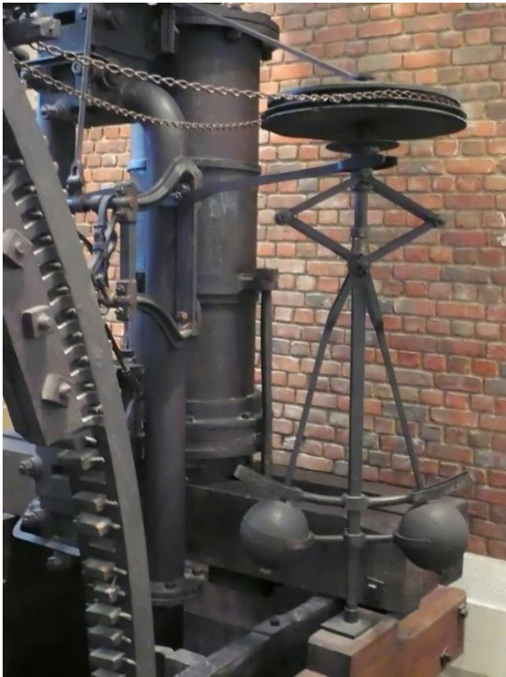
Figure 11 Watt's steam engine governor
