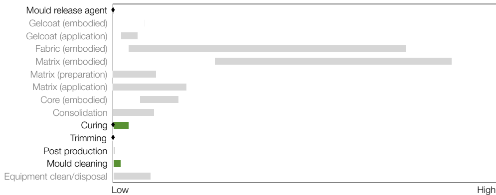
Figure 23: The relative impact and range of impacts for the remaining stages of composite product manufacture
