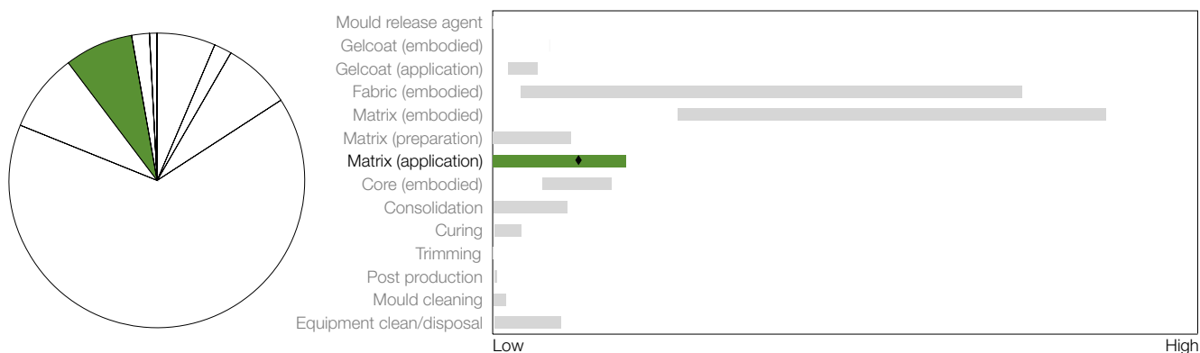
Figure 17: Pie and bar chart showing the relative impact and range of impacts of resin application. The pie chart and dot represent the impact of application by brush in the hand lay-up base case
