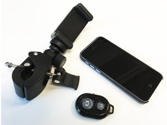
Figure 1: JourneyCam hardware, clockwise from left: clamp and phone mount; iPhone; Bluetooth trigger
