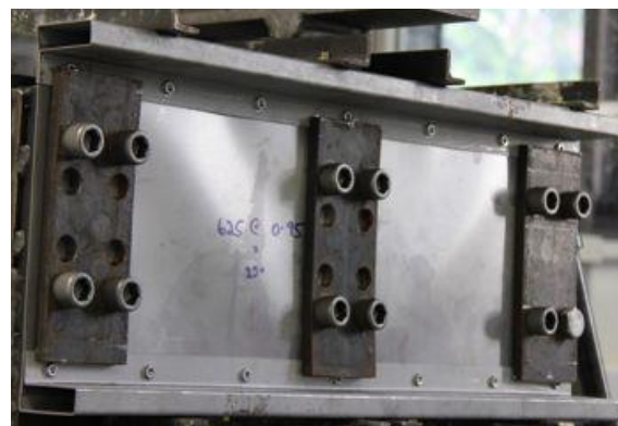
(c) 250x51x1.15x0.95 RHFCB (Test 7, AR of 1.0)
