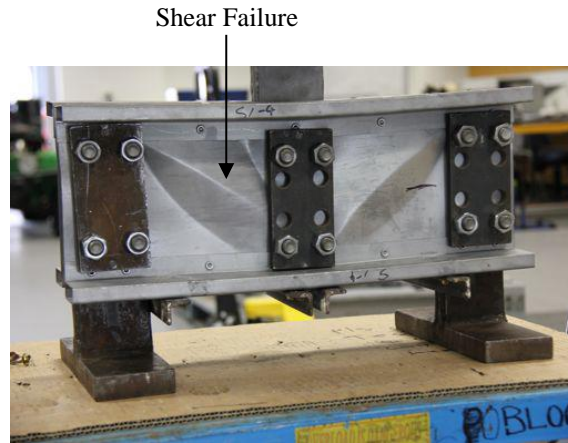
(a) 200x51x1.15x0.95 RHFCB (Test 5, AR of 1.0)
