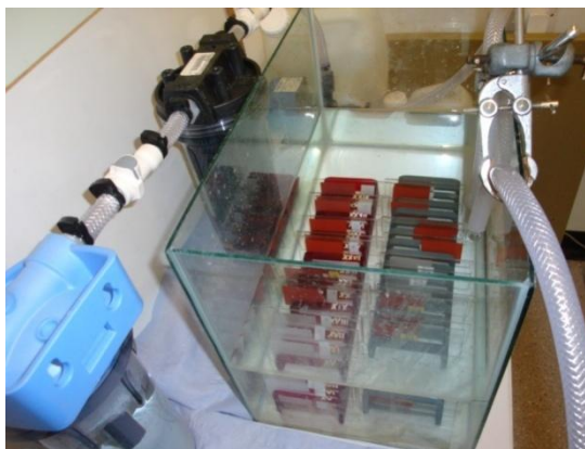
Figure 6:4: Photograph of leaching storage tank
