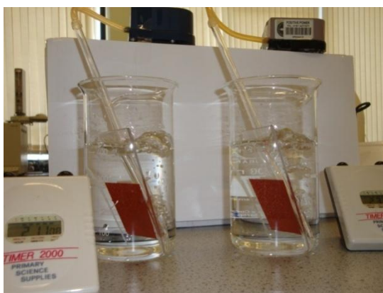
Figure 6:5: Photograph of a leach rate experiment using bubble agitation
