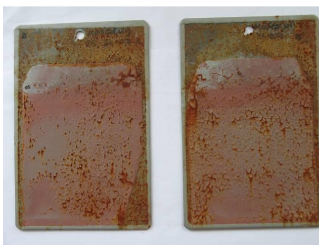
Figure 3:7: Photograph of MESQ(I)25 coating which failed after 6 cycles. The picture shows the corrosion of the coated steel substrate through the extensive cracking of the test coating.
