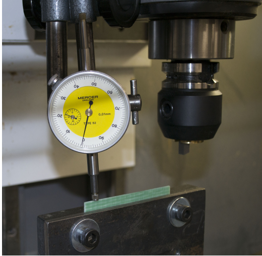
Figure 6.21: Dial gauge set up
