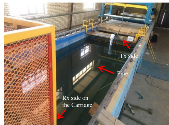
Fig. 2. Pipe installation exactly below the laser propagation path in a 12 m link span
