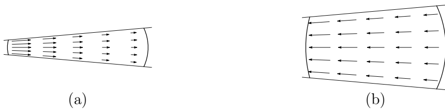
Figure 3.7: Pressure gradient force density, -\nabla p , for a barrel displaced (a) inwards and (b) outwards from the equilibrium position. The plots correspond to cross sections along the transverse plane, y = 0 . The displacements in (a) and (b) correspond to (X - X_e)/V^{1/3} = -1 and (X - X_e)/V^{1/3} = +1 . The contact and tapering angles are \theta_e = 110^\circ and \beta = 5^\circ .
