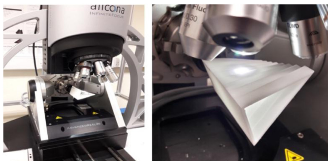
Fig. 6. Phase 1 – High resolution measurements with an FVM instrument. In this example, a TPU surface was measured.
