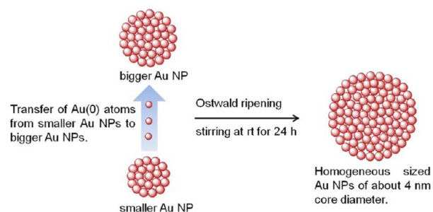
Figure 7. Ostwald ripening phenomena result in TOAB-Au NPs with a narrow size distribution. Smaller Au NPs in inhomogeneous population in terms of size dissolve and end up in bigger Au NPs.
