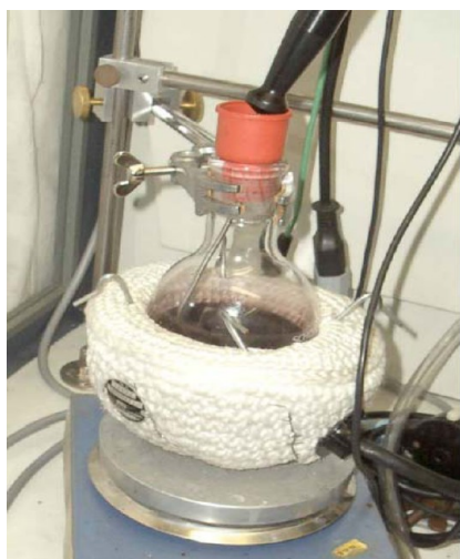
Figure 9. Au NPs are stirred after the addition of DDT while the temperature is controlled by a thermometer that is embedded in the reaction flask.
