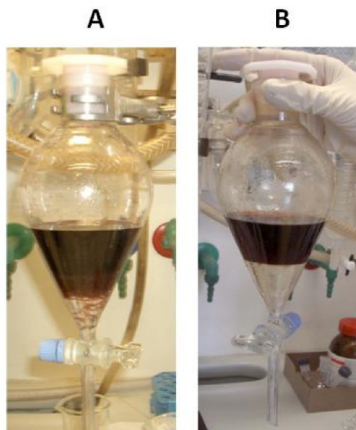
Figure 6. Purification of TOAB-Au NPs. Upper toluene phase containing TOAB-Au NPs is washed with aqueous solutions (HCl, NaOH, and Milli-Q water) in the lower phase to remove excess sodium borohydride and other residual chemicals. (A) Photograph of the two phases immediately after shaking: note that the two phases are not completely separated. (B) Photograph of the two phases after they were allowed to separate, forming a transparent aqueous phase at the bottom and a deep red organic phase at the top containing TOAB-Au NPs.
