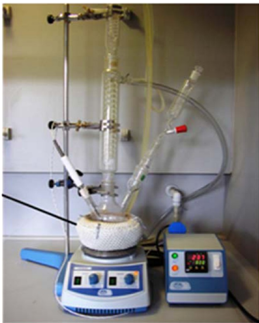
Figure 19. Setup for the synthesis of CdSe/ZnS NPs. The photo shows a three-neck flask equipped with a heating mantle, a reflux condenser, an addition funnel, a thermometer connected to a temperature controller, and a nitrogen flow.
