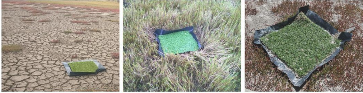
Figure 3.2: Astroturf mats were installed across the Droë River wetland to measure the rate of short-term sediment accretion.
