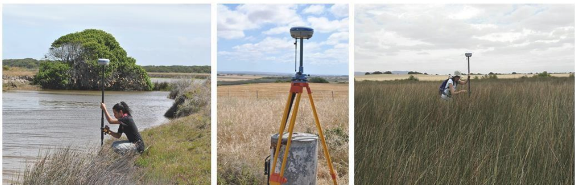
Figure 3.5: A detailed DGPS survey was conducted within the wetland. The survey captures the morphology of the wetland, in some areas, the old river course can be seen.
