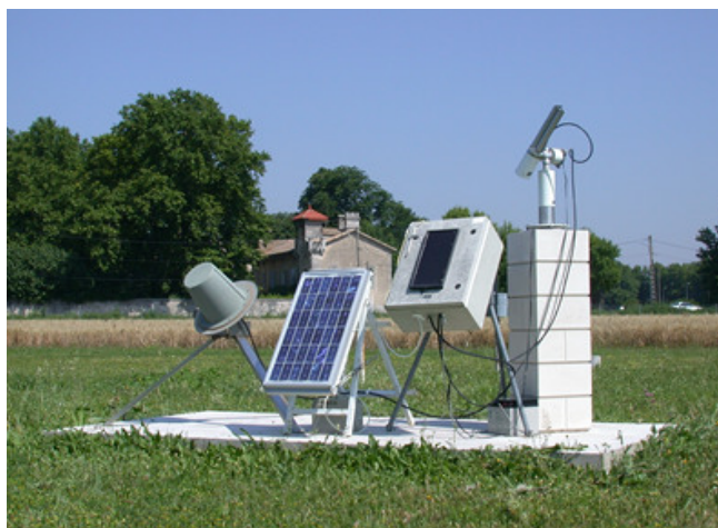
Figure 2.3 CIMEL Electronique CE-318 sun-sky radiometer used by AERONET (Source: NASA Goddard Space Flight Center, n.d.)
