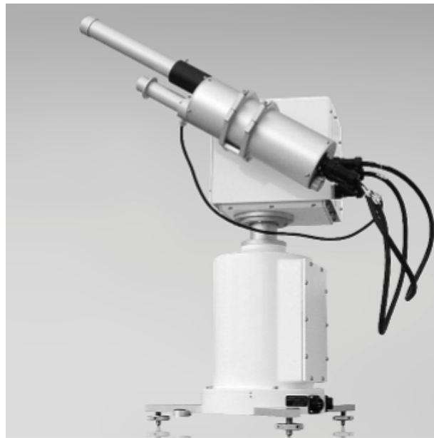
Figure 2.4 PREDE-POM sky-radiometer adopted by SKYNET (Source: Pre-TECT, 2016)
