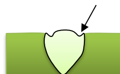
Figure 16: Illustration of the undercut defect.
