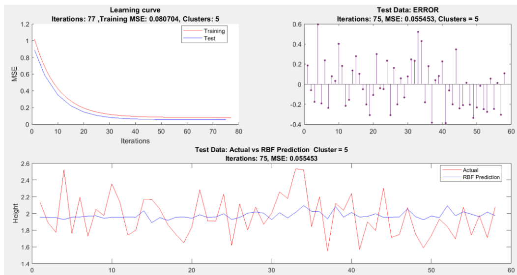
Figure 91: Illustration of the result of RBF training with learning rate of 0.0003 and 5 cluster centers.
