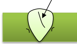
Figure 15: Illustration of the crack defect.
