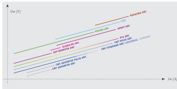
Figure 11: Illustration of current and voltage diagram of CMT in different modes [30].
