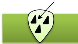
Figure 20: Illustration of the slag defect in welding.
