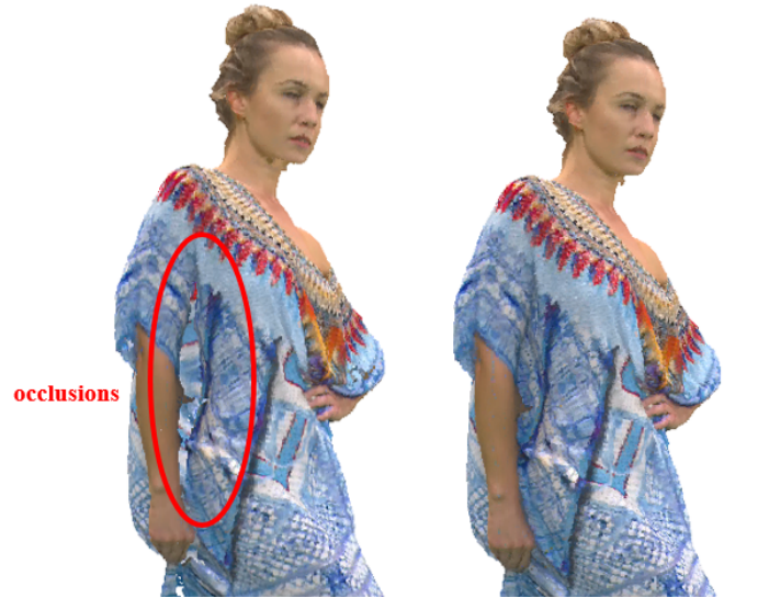
Figure 3.16 Sequential decimation improves the occlusion handling in some concave areas (left)
