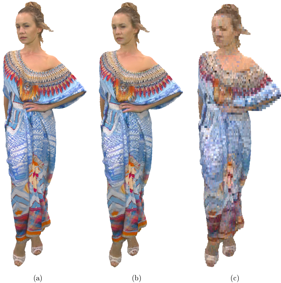
Figure 2.2 (a) Original point cloud (b) decoded point cloud at 13 Mbit/s for proposed solution, and (c) reference technology [1]
