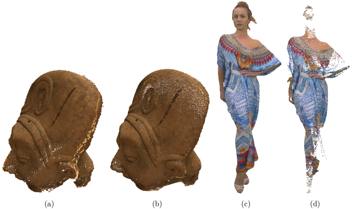
Figure 3.8 (a) Original Egyption point cloud (b) reconstructed point cloud in sphere projection (c) Original Longdress point cloud, and (d) reconstructed point cloud in sphere projection
