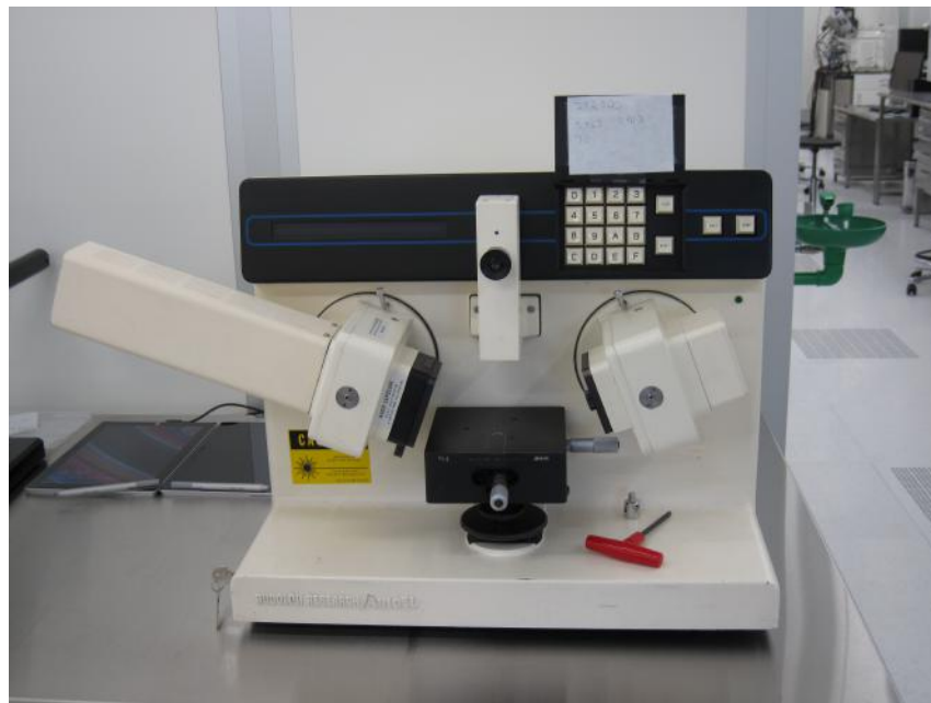
Figure 3.7 The Rudolph Auto EL III Ellipsometer that was used in ellipsometric measurements.
