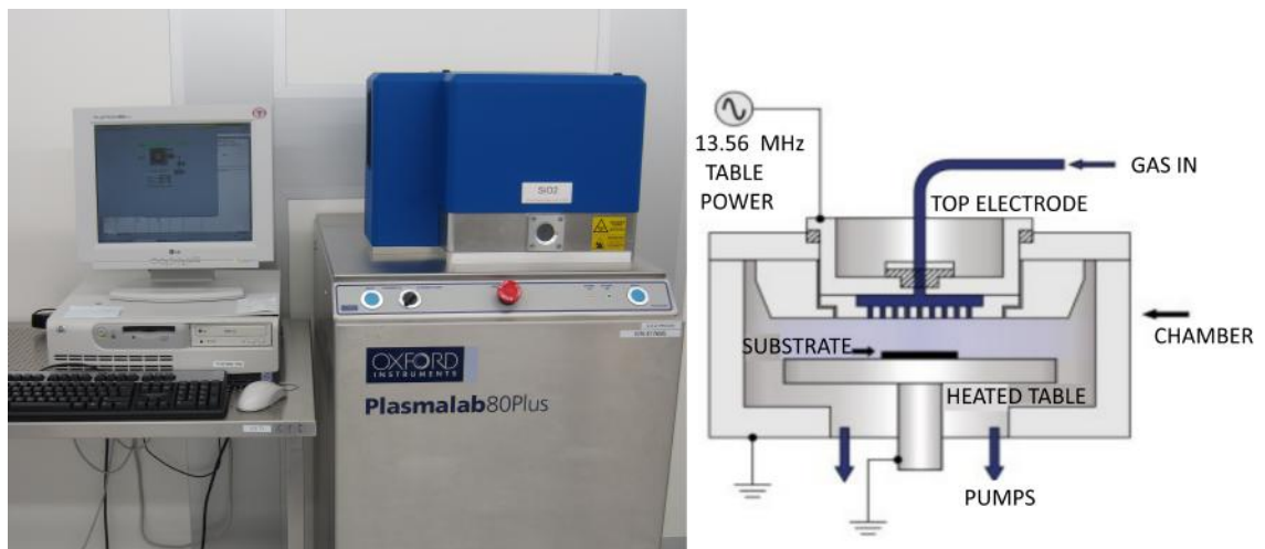
Figure 3.2 At left the plasma enhanced chemical vapor deposition system in the cleanroom at TUT and at the right the illustration of the used PECVD system applied from [115].
