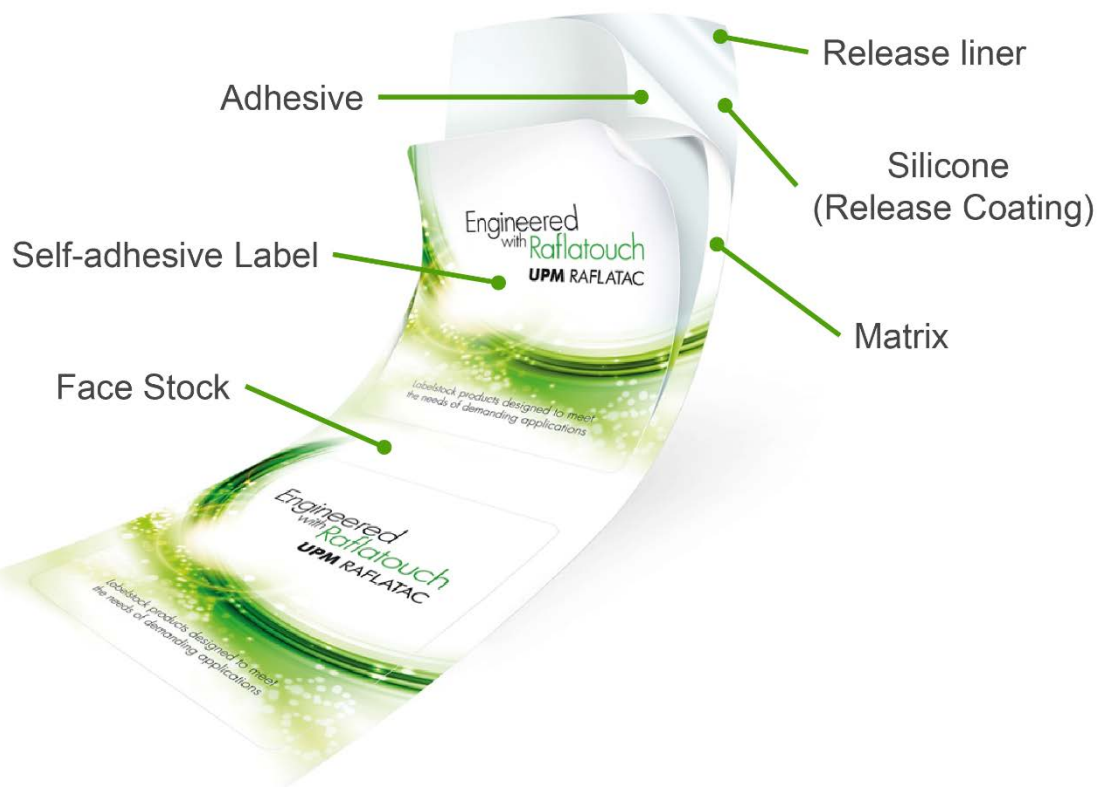
Figure 2. Components of the “Engineered with Raflatouch by UPM Raflatac” PSA. [5]
