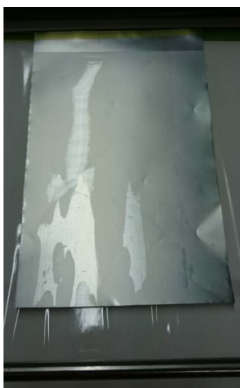
Figure 24. Uneven silicone coverage of the aluminium sample sheet as not enough pressure was applied to the coating bar.
