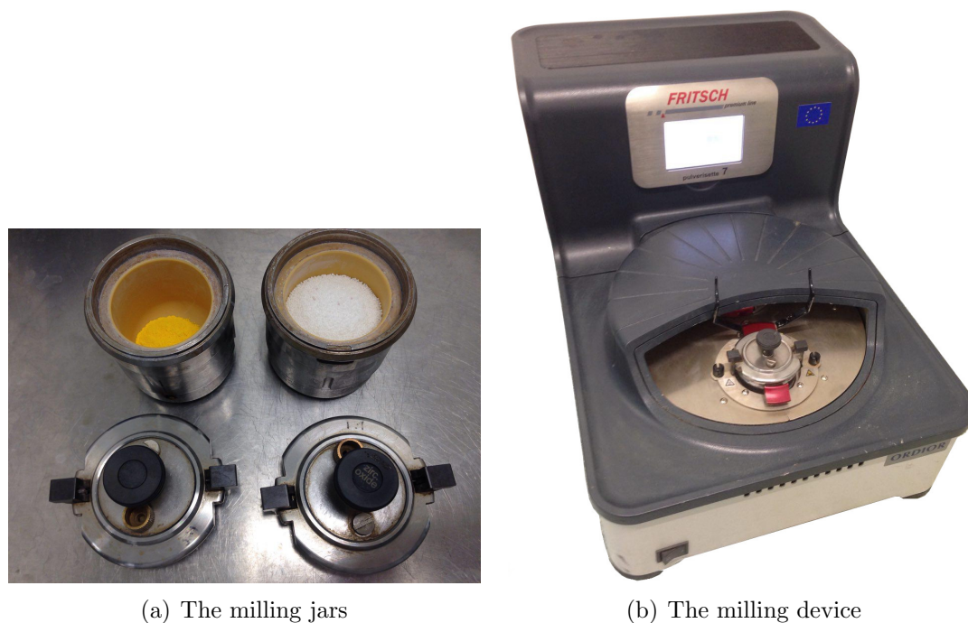
Figure 4.1: The milling system comprises (a) the milling jars and (b) the milling device (Planetary Micro Mill Pulverisette 7, Fritsch GmbH). The yellow powder in the jar on the left side is bismuth oxide and the milling balls are in the jar on the right side.
