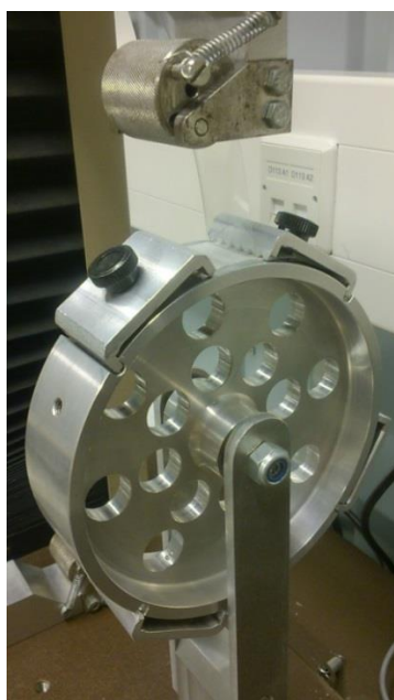
Figure 23. The setting for peel test done in 90° peel angle.
