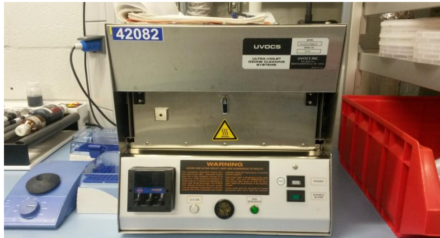
Figure 13. UVOCS® ultra-violet cleaning machine
