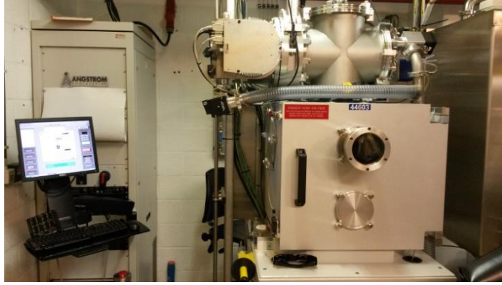
Figure 17. Angstrom system used for deposition of gold contacts
