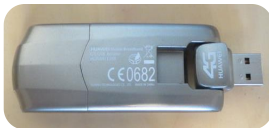
Figure 4.2. Huawei E398 LTE USB modem used as the UE.
