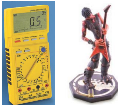
Figure 3.14. Multimeter prototype (left) and figurine (right) created using ZPrinters from 3D Systems, Inc. (3D Systems, 2012c).
