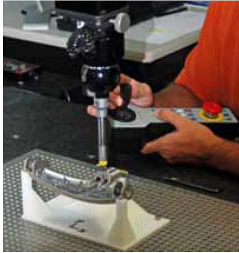
Figure 3.11. A fixture (the white part) made with FDM technology (Hiemenz, 2012).
